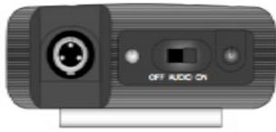
You'll notice there's also an on/off switch on the top of the unit. Don't get that confused with the power switch (people do it all the time... including the audio guy at my wedding!). This top switch is just a "mute" switch for the microphone. It lets the microphone wearer turn the mic on and off without affecting the transmission.
